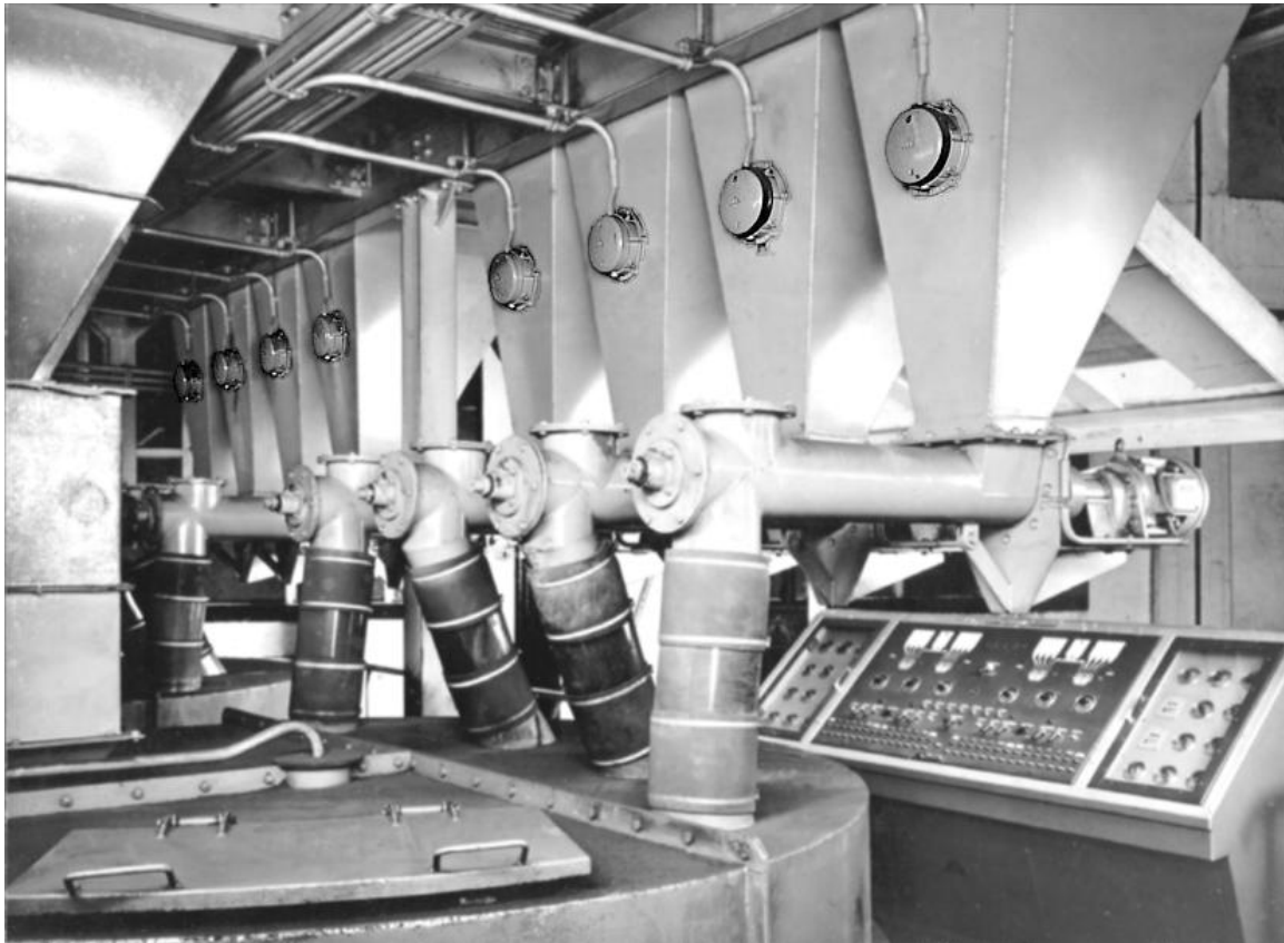
Pictuer: Fill level monitoring in silo outlets of an automatic processing plant
